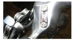
The travel range of a derailleur is determined by Limit screws and the chain's world is confined to a zone within these Limits. The logic seems simple. The Limit screws are there to save the chain from falling off the cogs. We set the outer Limits to allow the chain to safely travel over the 10 or 11 cogs without falling off the edge and then forget about the Limit screw – because it has done its job.
