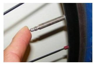
The **V**alve on the inner tube of a tyre is an amazing invention. It lets air in and that air stops itself from escaping by pushing back against the valve. The only way that air can be released is by an external power source that forces the valve open.
