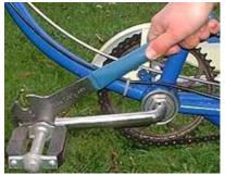
The guy at the bike shop had no such trouble. One firm push with the Pedal wrench and the bloody left Pedal spun off! "It is a left hand thread" He said. "It unscrews the other way..." Now I know that the left Pedal has to defy convention to make it stay on the crank arm. If it was a conventional right hand thread, the friction of the pedaling action would unscrew the Pedal.
