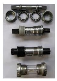
The old square taper axle **B**ottom **B**racket assembly has now been replaced by a multitude of alternatives. There is "octalink", "ISIS", "Hollowtech", "Ultra toque", "BB30", "BB90", "Press fit" and others. The bearings are "inboard", "outboard" and anywhere in between. The axle lengths and shell widths also vary. Then there is the English or Italian thread.
