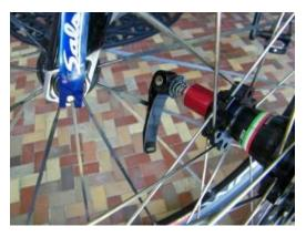
In the old days, bicycle riders had to carry spanners to undo the wheel nuts when a wheel or tyre change was needed. Then someone invented the **Q**uick release and the simple action of a cam revolutionised the wheel change. One swing of the **Q**uick release lever and the wheel 'drops out'.
