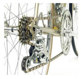
On our bikes we have a front **D**erailleur and a rear one. They both instigate a gear change – but in two totally different ways. The front **D**erailleur simply gives the chain a push and lets go. It then stays out of the way. The rear **D**erailleur does it quite differently. It never lets go of the chain. Instead it provides the chain with continuous guidance – as it pulls the chain across the gear cluster.
