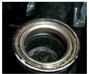
With sealed bearings, simplified housings and stem, Headsets have improved and the worn headset is not as common nowadays. In the past, they used to have ball bearings rolling around in retainers. The balls used to wear into the cups and create pits in the bearing races- locking the front forks into the 'straight ahead' position.
